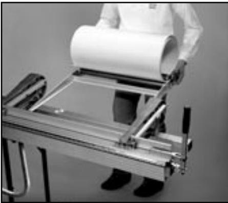
Hooks on and detaches in seconds. Allows you to roll out and cut coil squarely to your exact length.
