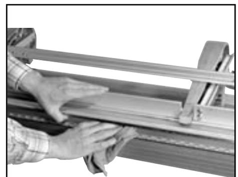
**6 Clean Underneath Clamping Surfaces**
